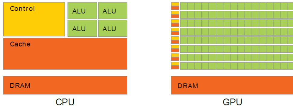
Figure 1.8: Schematic comparison of CPU and GPU architectures. Image from *NVIDIA*<sup>6</sup>.
